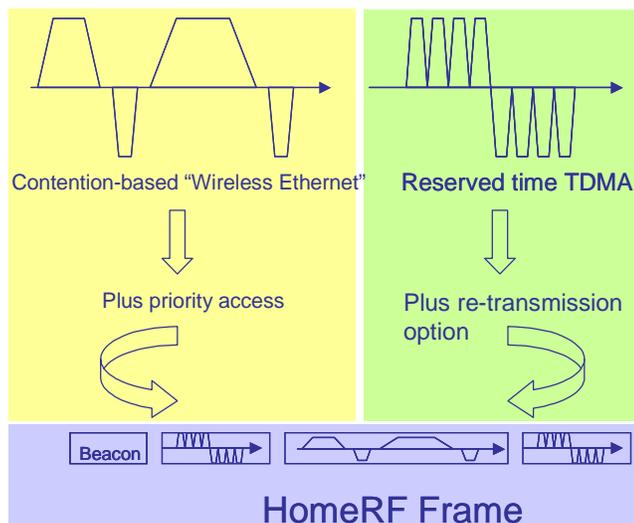
**Figure 5: Basics of the HomeRF MAC Frame Structure**
