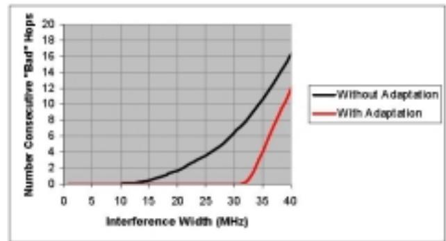
**Figure 18: Performance of the HomeRF Hopset Adaptation Algorithm**
